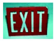
There are a couple ways to know whether an EXIT sign contains tritium. When the lights are off, tritium will make the word EXIT glow green or red. The sign should also have a permanent warning label that mentions tritium, 3H or H-3; displays the three-bladed radiation warning symbol; and states "Caution-Radioactive Materials." If all four letters in EXIT are fully lit, the sign is working properly. If not, the sign may be damaged or have reached the end of its working life.
