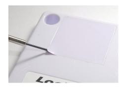
1.2 Turn battery door anti-clockwise and remove from case.
