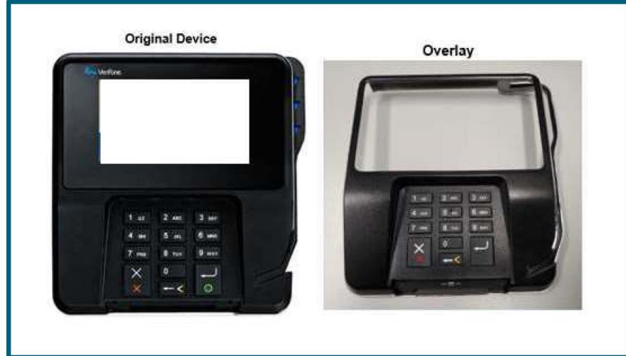
Device overlays are usually put in place with double-sided tape to adhere to the original machine. The skimming overlay can easily be removed by lifting the edges or corners, this will allow the overlay to separate from the original device.
